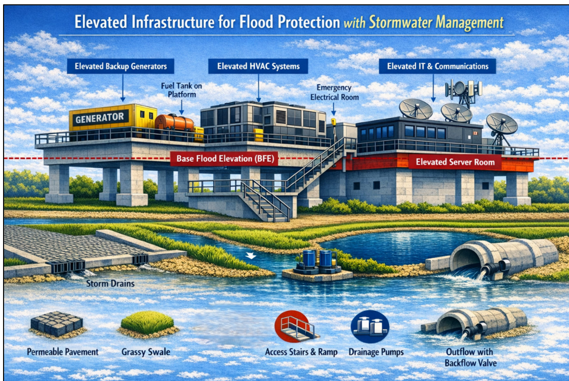
Figure 5: Examples of Site-Level Flood Protection Stormwater Retrofits
