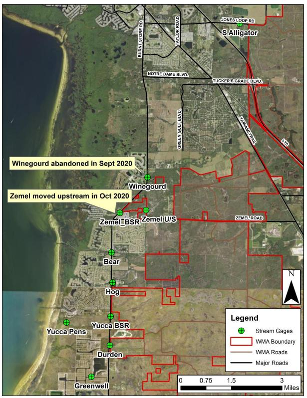
Figure 2-2. Flow Monitoring Stations
