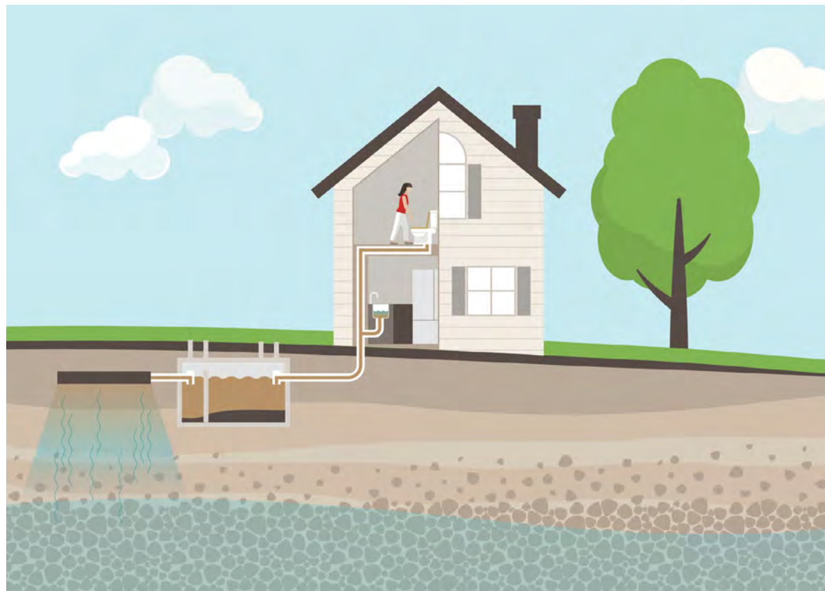
▲ Figure 12. Conventional residential septic systems are currently designed to treat bacteria. Because they only treat 30–40% of nitrogen input (Toor et al. 2011), they can be a source of nitrogen pollution in the watershed | www.ourwatershed.ca .
