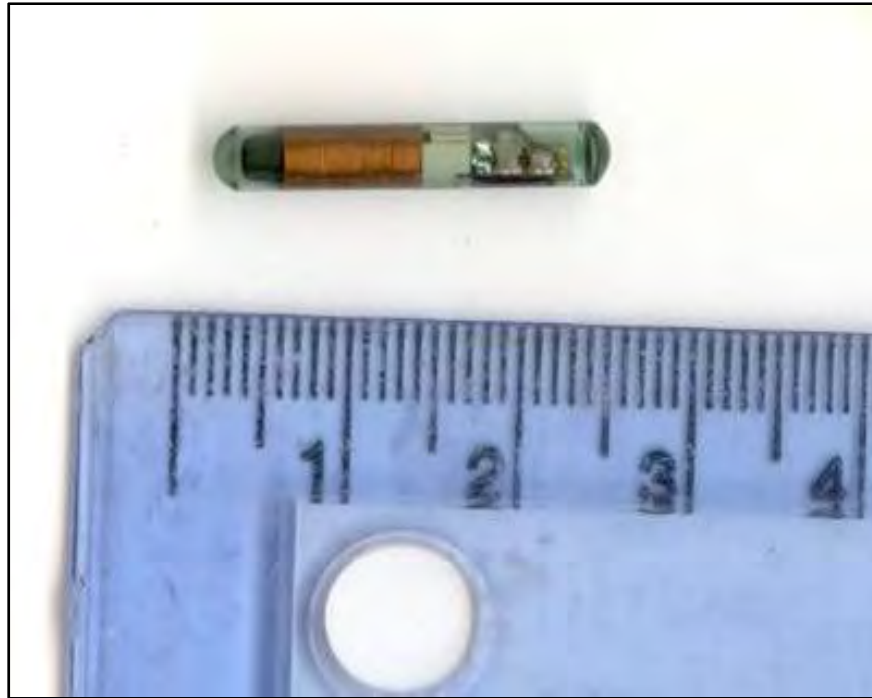
Figure 2. PIT tag used for tagging juvenile tarpon.
