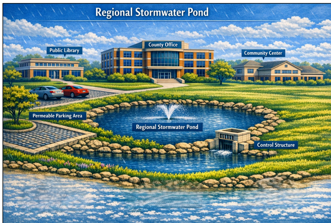
Figure 7: Example of a Regional Stormwater Management System
