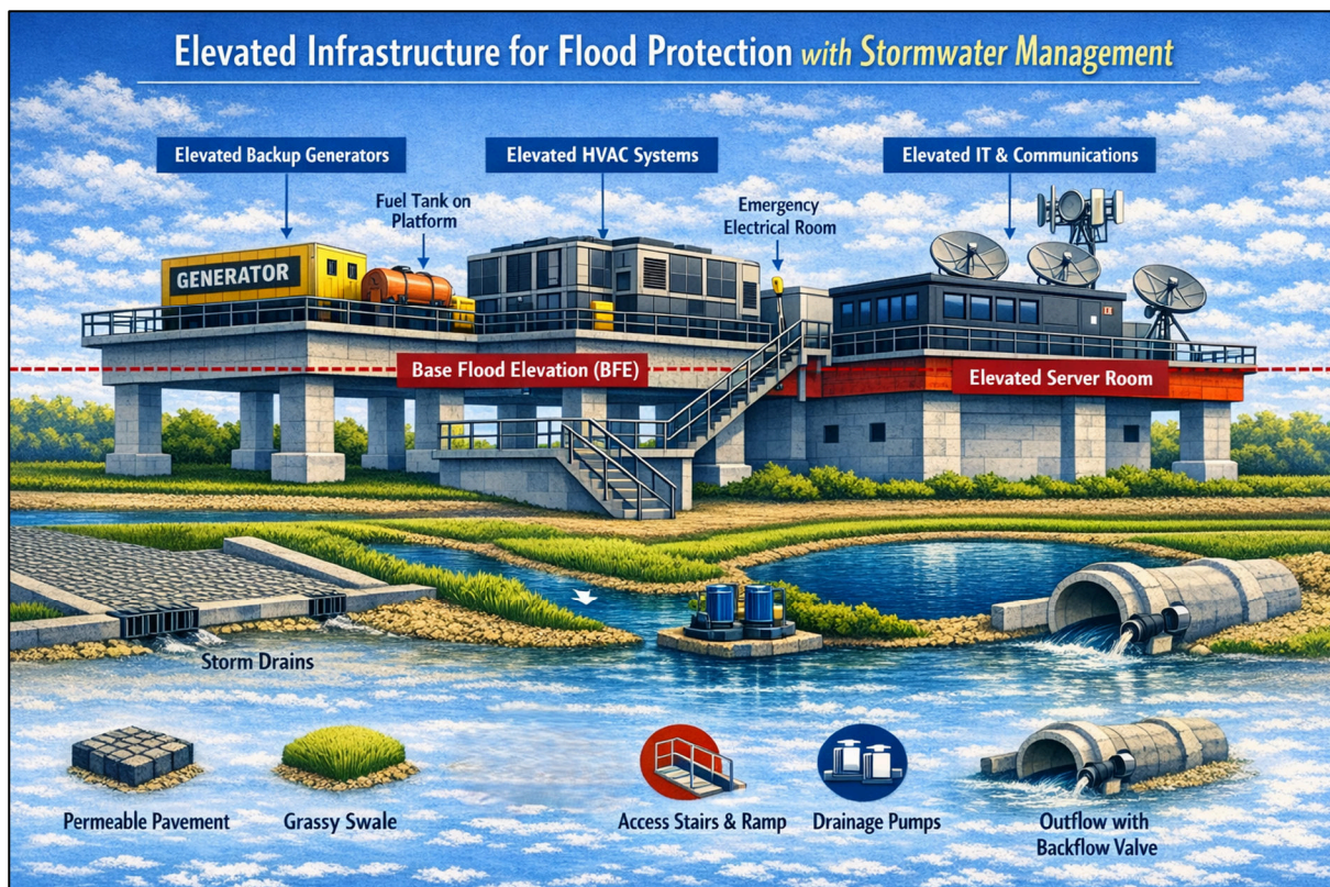
Figure 5: Examples of Site-Level Flood Protection Stormwater Retrofits
