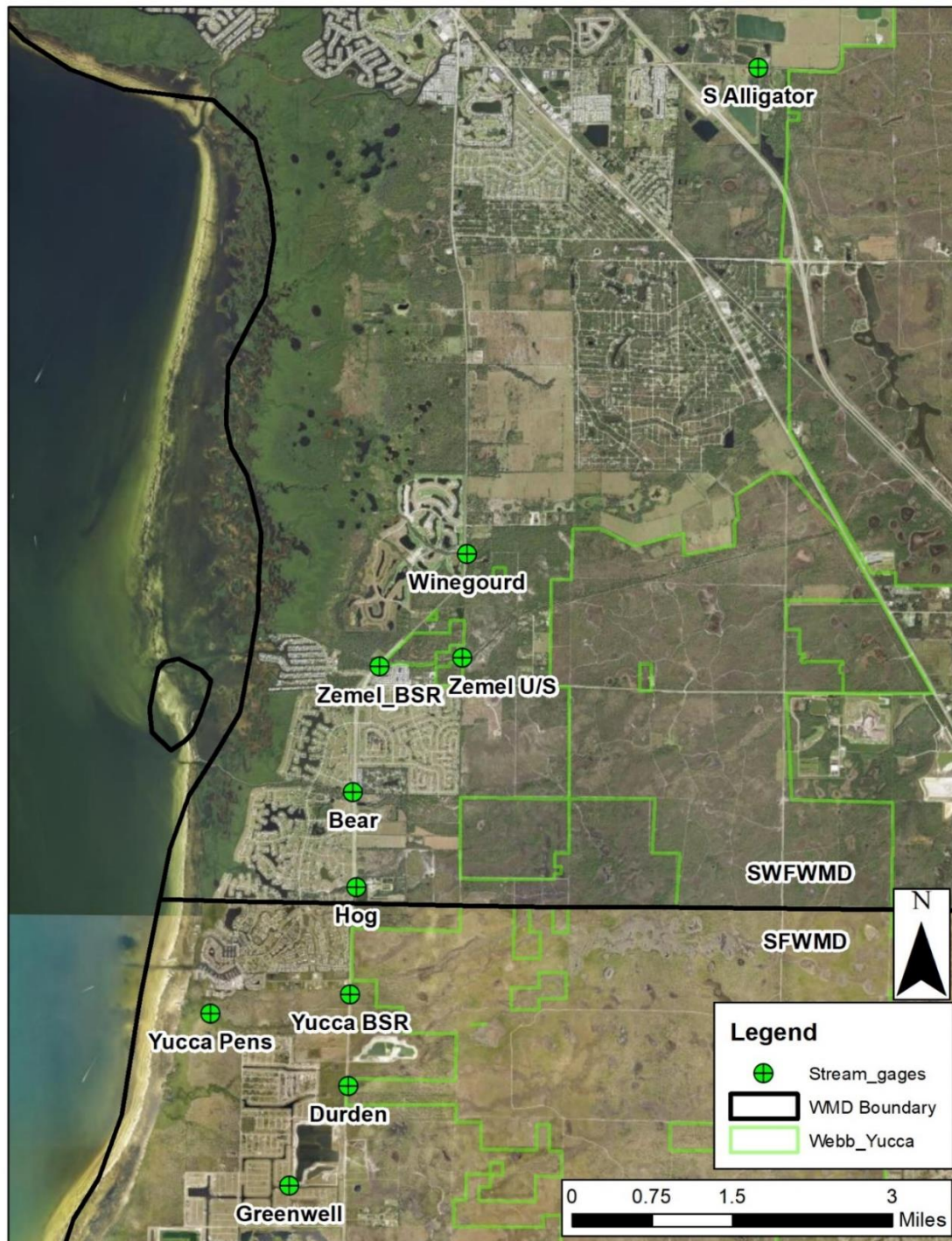
Figure 1 - Flow Monitoring Stations
