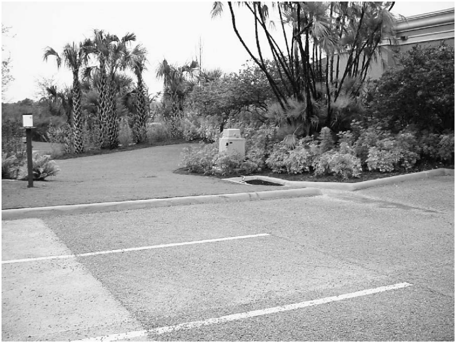
FIG 3. Pervious Pavement Study at Shadow Wood Preserve showing the inlet and sampler.
