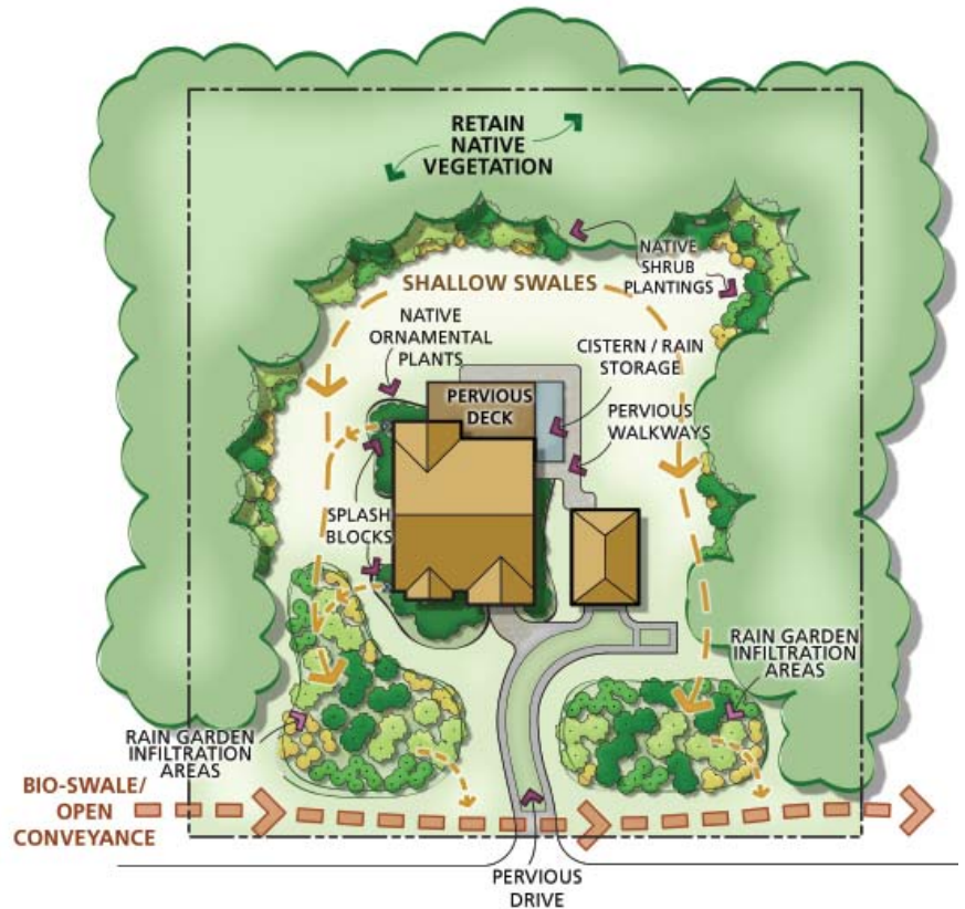
Low impact development (LID) practices, many of which are shown above, reduce stormwater runoff and reduce the need for large regional stormwater treatment systems.
